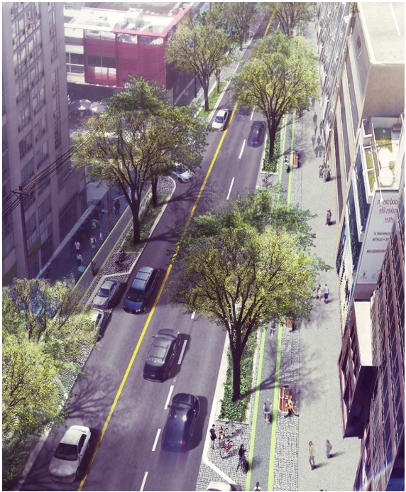
Example of bikeway and parking bump outs, proposed for Eglinton Ave. (Midtown Yonge Study)
